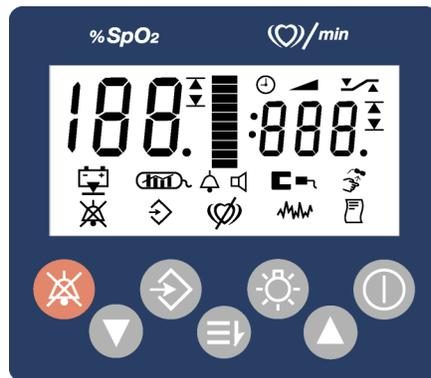
**%SpO<sub>2</sub>** Displays the measured percent of oxygen saturation.
